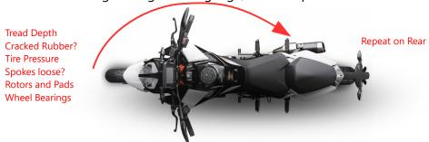
**C – Controls** Get on the bike. Without starting the bike, turn on the ignition key. With the front brakes applied, lean forward and backward to compress the forks. Rotate the bars when doing this. Release the front brakes and apply the rear, repeat. This will test both brakes, levers, suspension, and steering head bearings with one quick action. Clunk = Junk.
