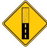
Pavement ends Continuation has gravel surface
