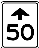
Advance warning of a lower maximum speed zone ahead
