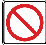
Signs with a red circle and diagonal slash deny permission, as indicated
