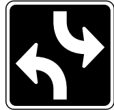
Two-way left turn lane
